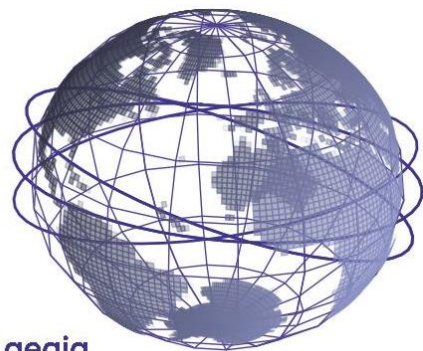
Figure 1. A depiction of 3 satellite orbits around the Earth produced by Atlas for the NATO constellation. These orbital trajectories offer maximal coverage of NATO sites in Europe and North America.
