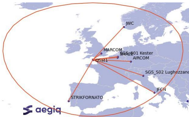
The free-space line of sight of a Low Earth Orbit satellite flying over western Europe, with links to ground stations highlighted
