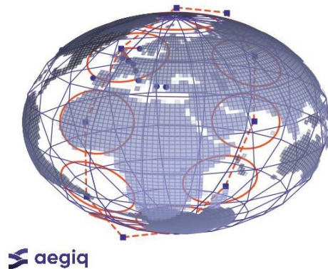
Visualisation of a Low Earth Orbit constellation of 9 satellites and their line of sight footprints as they traverse the globe
